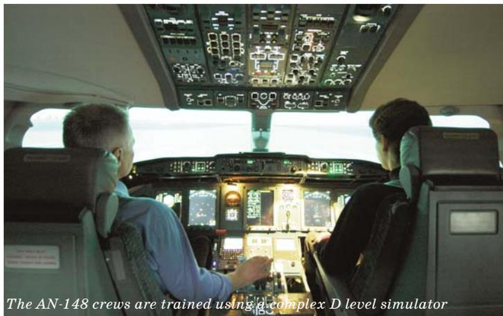
*The AN-148 crews are trained using a complex D level simulator*
